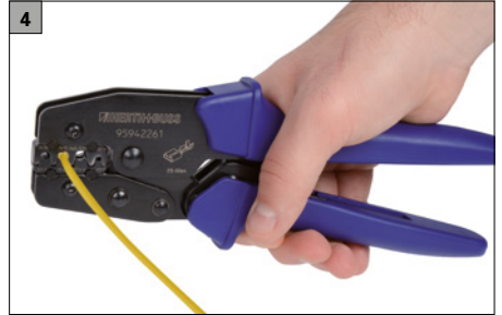
4 Close the tool until it opens automatically.
