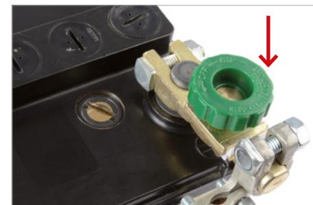
Now mount the quick breaker clamp onto the negative terminal along with the negative clamp which was just fastened to the bolt.
