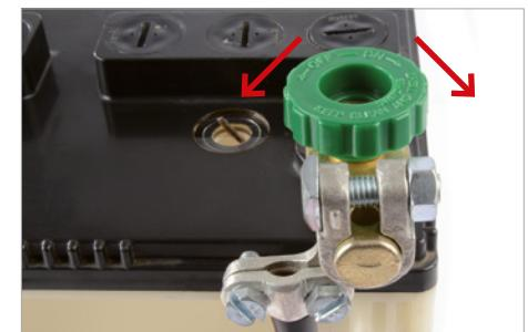
The circuit is closed by tightening the knurled screw fully in the direction "ON". Two to three rotations of the knurled screw in the direction "OFF" are sufficient to interrupt the circuit.
