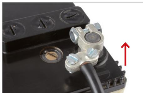
Remove the battery terminal clamp, which is currently connected at the negative terminal, from the terminal.
